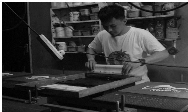
Gambar 5. Proses sablon manual
